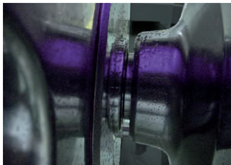
Riboflavin Test - after CIP
