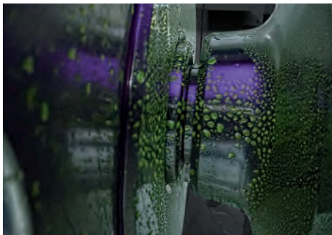
Riboflavin Test - before CIP
